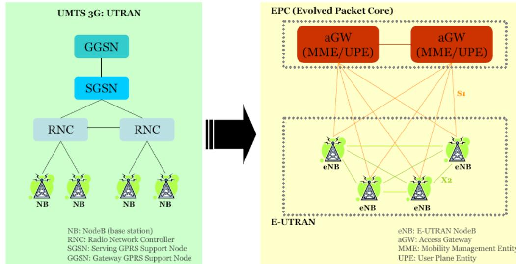
The **removing of RNC network element** and the **introduction of X2 interface for direct communication between the eNodeBs** makes the radio network architecture **more simple and flat**
