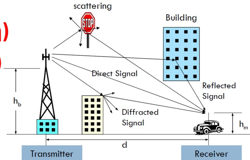
**Reflection, Scattering and Diffraction leads to Multipath Propagation!**
